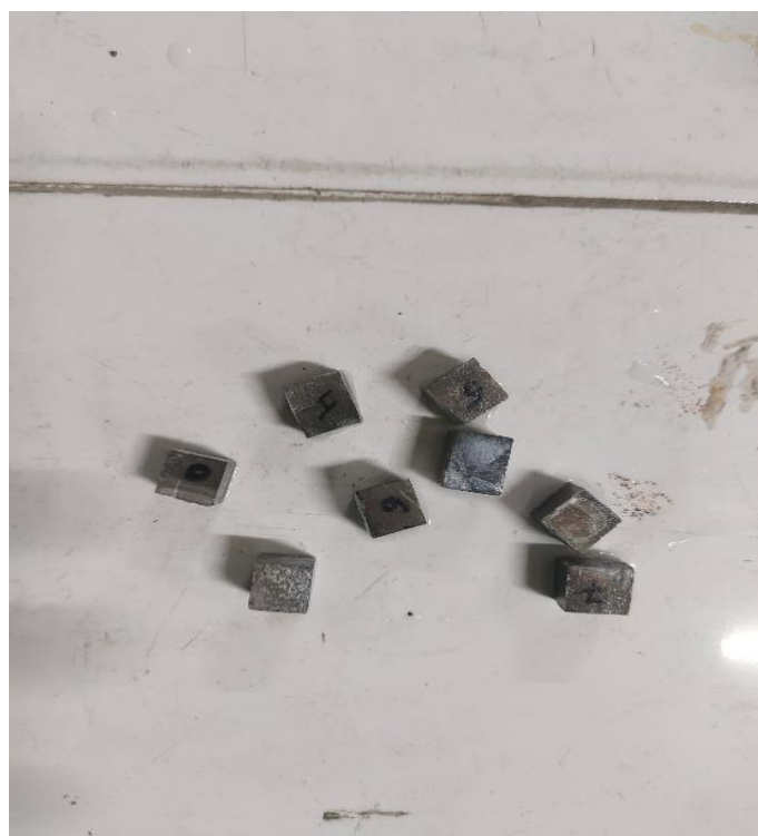
Fig. 3. Representative Images of Composite Samples After Immersion in 3.5% NaCl Solution.
